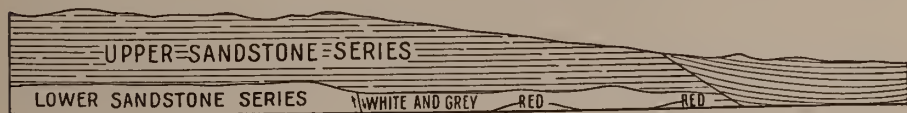
FIG. 175—Sketch section to show the structural details of the strata on the south wall of the Majes Valley near Cantas. The section is two miles long.
